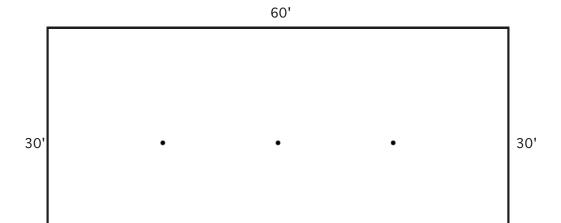
The linear feet of a tent's perimeter is the sum of the 4 sides of the tent. In this example - based on a 30'  $\times$  60' tent - there is 180 feet around it's perimeter
